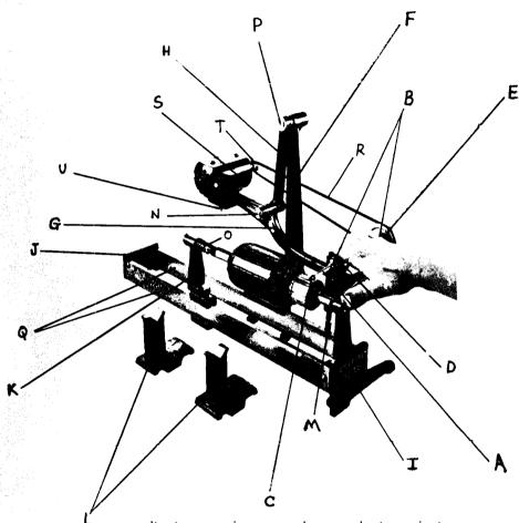
Its two moving arms have only two pivots, making operation exceedingly easy. Sturdy one piece cutter-spindle, rotated with one belt to motor.
